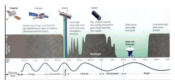
Figure 2. Atmospheric absorption of power over many wavelengths. Notice the depth of the transmission windows around 12cm vs  $1\mu$ .
