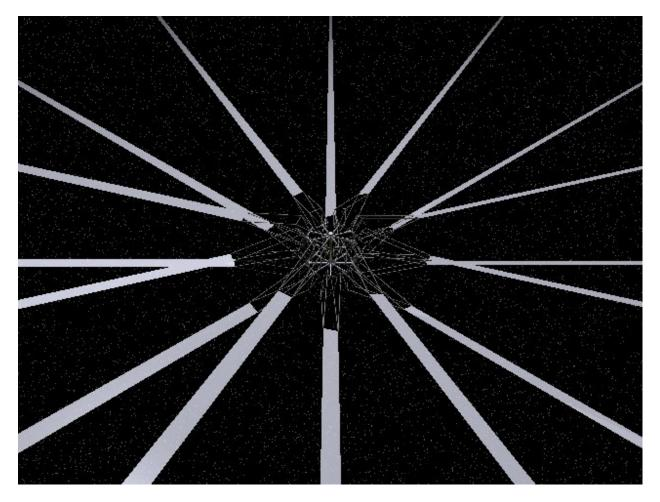
Figure 3. Artist conception of the JPL heliogyro Halley's Comet spacecraft design. Note multiple layers of blades. Image courtesy of CalTech.
